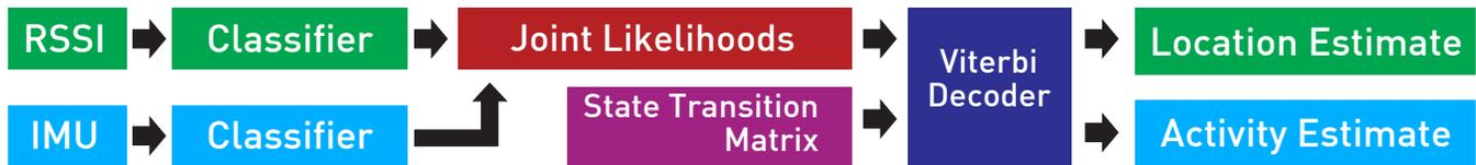
Figure 1: System data flow showing how IMU and localization data are combined into joint likelihoods which are evaluated by a Viterbi decoder using a joint state transition matrix.
